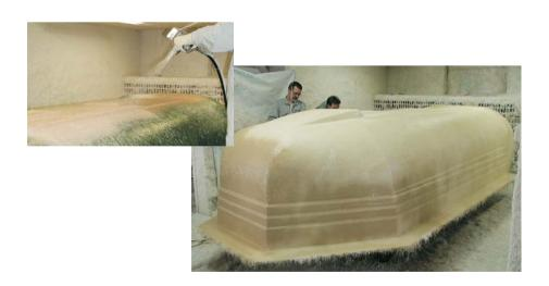
The new generation of **Polylite® 33542 Profile Tooling System** allows for easy tool manufacturing and excellent performance during practical use. In case you need advice on application and layout, feel free to contact your Reichhold representative.
