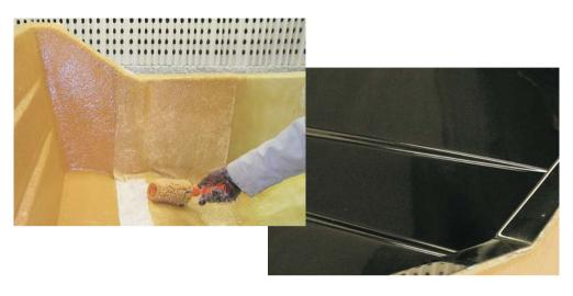
Time for de-moulding from the plug is typically 24 hours at room temperature.
